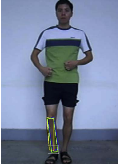
Fig. 10. This figure indicates the result of projected right leg block on the image plane under three joint candidates and determination of the expect one by local search. The dot rectangle indicates the search region, the red dot indicates the search center, and the green dot is the expected location of the joint. The corresponding Euler angles are estimated as the pose of this joint. (For interpretation of the references to color in this figure legend, the reader is referred to the web version of this article.)
