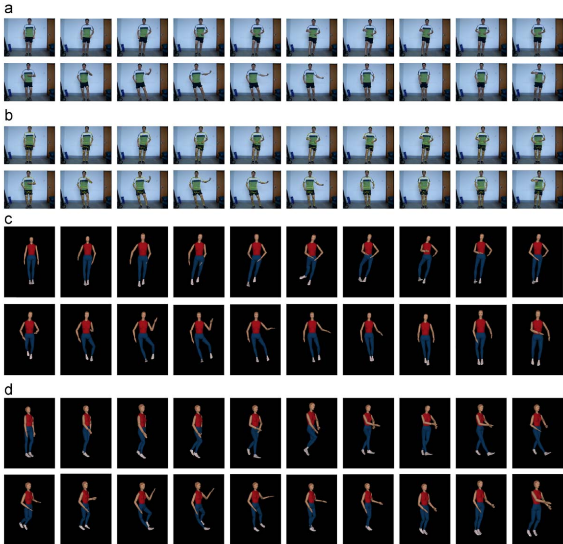
Fig. 14. Results of reconstruction of 3D human pose from the test video sequences in which the subject's left arm moves in a decreasing spiral (every 15th frame from 15 to 300 arranged from left to right, top to bottom). (a) Tracked frames. (b) The projection of expected model configuration on the original images. (c) Reconstructed human poses from the front view. (d) Reconstructed human poses from the side view.
